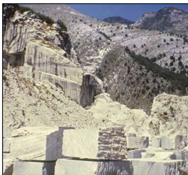
Figure 8. An older image of stacked marble blocks that had been cut out with wire-saws and the use of line-drilling.
