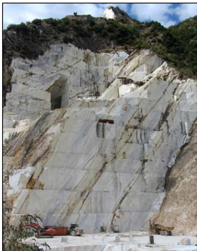
Figure 5. High wall of the Crestola quarry, with steeply dipping bedding features crossed by the working benches.
